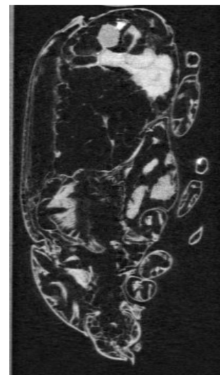
Figure: CT of a ground beetle, acquired using a lab-based EI setup with the new single-shot method (acquisition time <7').
