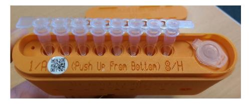
Use holes on the side to hold the PCR strip whilst pipetting samples in.
