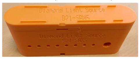
Remove the lid by prying underneath the cut-outs at the side
