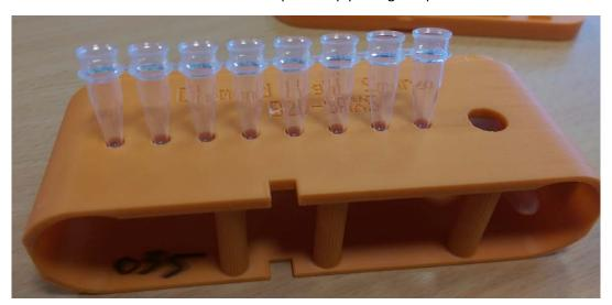
If the samples are for the Robot (Batch mode) remove Eppendorf from container and fill with 1.5ml matched buffer.
