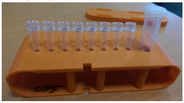
Align the tubes in the holder with the numbers on the tubes corresponding to the numbers on the holder 1 through to 8.
