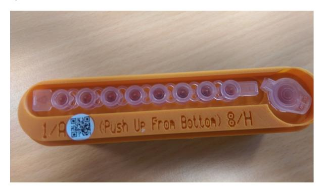
Place a zip tie in the cut-out at the bottom of the holder in this orientation and secure the holder by fastening the zip tie. A 4.6mm zip tie should fit well.
