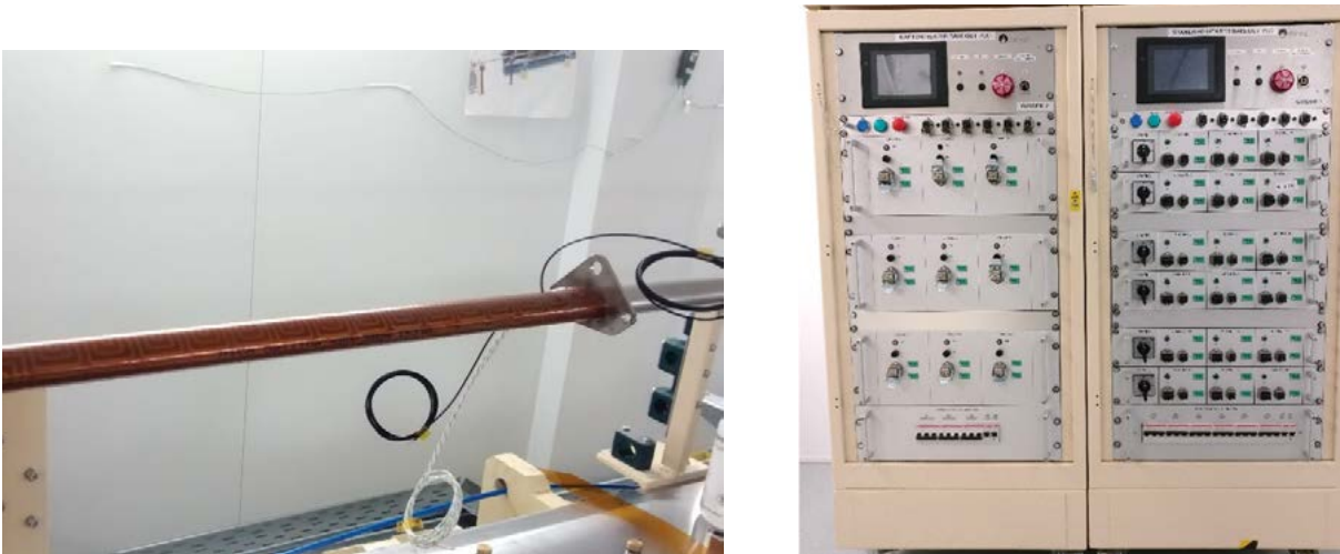
Figure 2-123 : Left - DDBA vessel with thin film Kapton heater applied; Right - PLC-based bakeout controller developed for DDBA.
