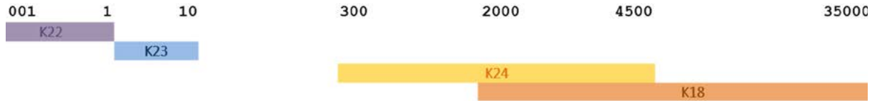
Figure 2-5: Energy range for the four BM beamlines considering adopting a 3PW as a radiation source.
