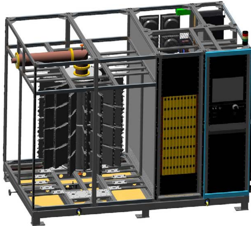
Figure 2-146 : High power solid state amplifier schematic.
