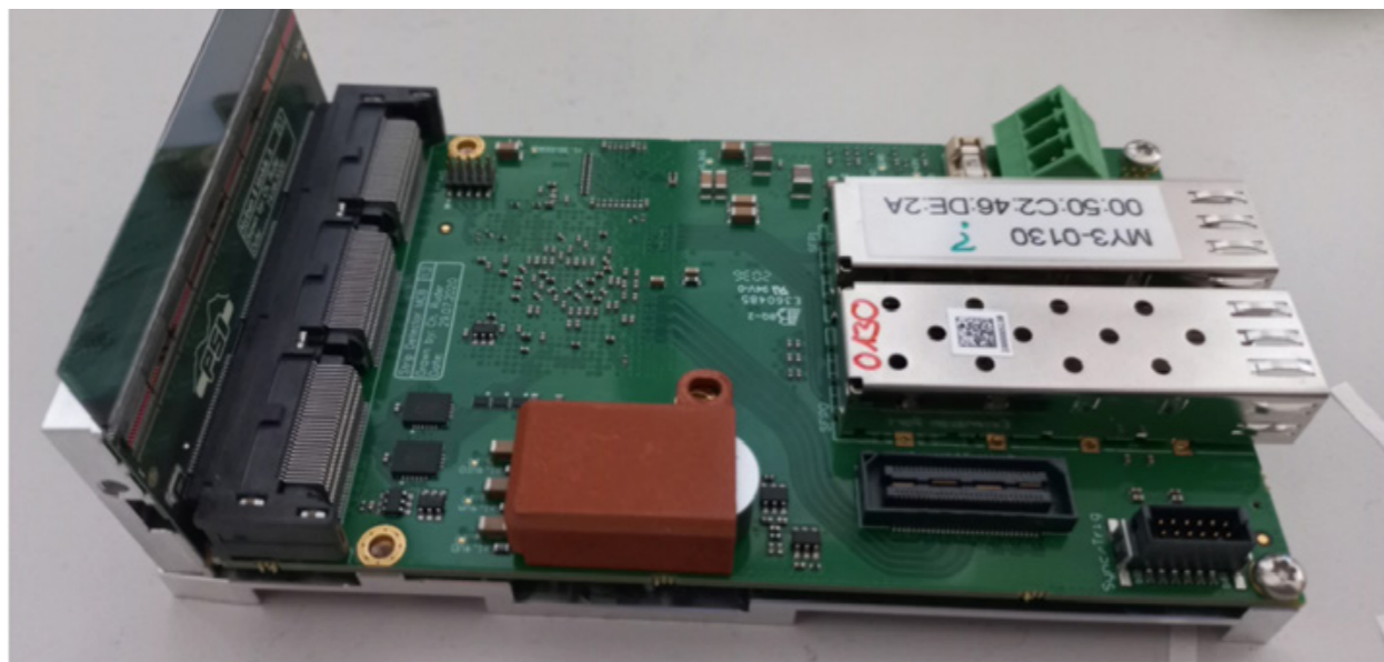
Picture of the Mythen III detector module ready for acceptance testing in preparation for the I11 PSD upgrade. The module is composed of 1280 independent channels acquiring in parallel in single photon counting mode, each connected to a strip of the silicon sensor (shown on the left of the image).
