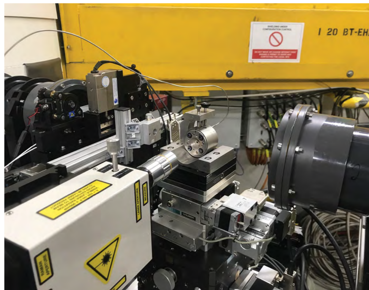
Figure 1: DAC installed on the I20-EDE experimental hutch.
