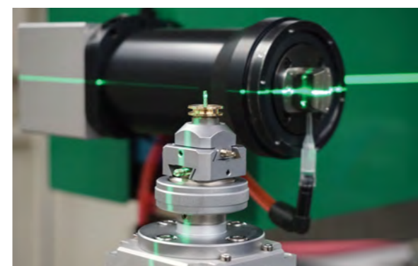
Figure 5: Sample being aligned on DIAD beamline (green light is sample alignment laser).
