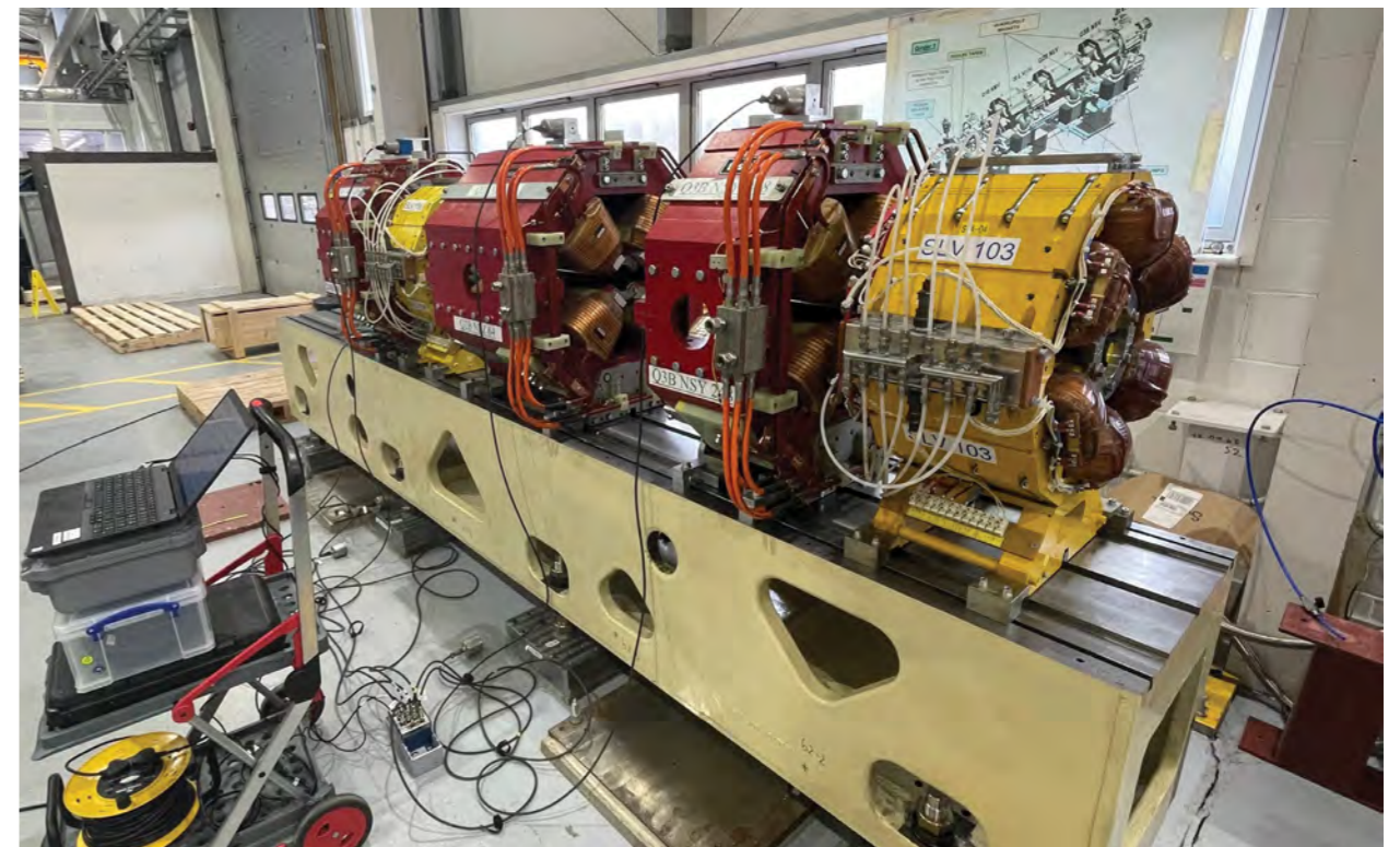
Figure 4: Testing new girder materials for their vibration performance for Diamond-II.
