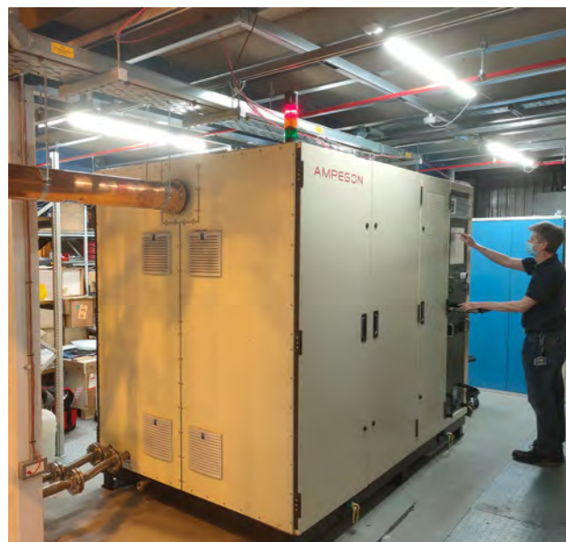
Figure 2: Diamond's first 500 MHz solid-state amplifier (left) powering the third normal conducting cavity in the RF Test Facility (right).
