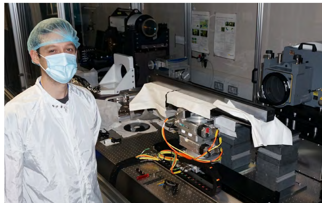
Figure 1: Murilo De Bazan, Metrology Scientist, with the Fizeau interferometer stitching system built at Diamond.
